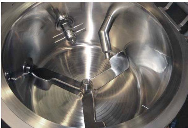
Mixing chamber with chopper and spraying system
