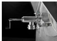
Discharge for taking samples – also under pressure or vacuum
